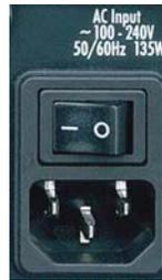
Figure 12 – Master Power Switch and AC Power Input
